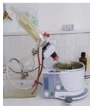
Fig. 3 Rotavapor type R3000-Gemini BV for the distillation of extracted oil
